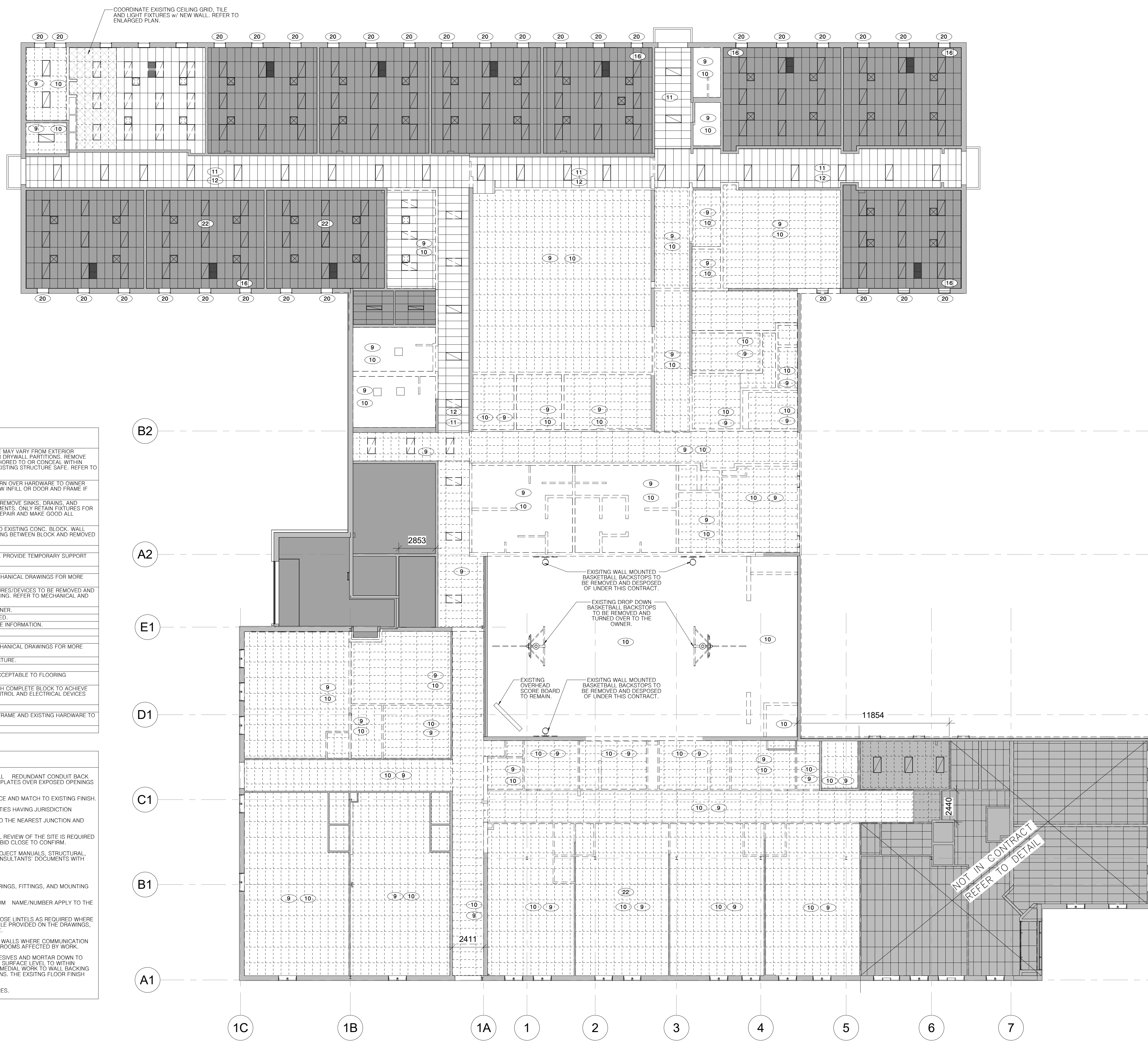
1 REFLECTED CEILING DEMO PLAN SCALE 1:150
